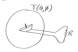
For  $T(\theta, \phi) = T = constant$ Resistor R > temperature T
